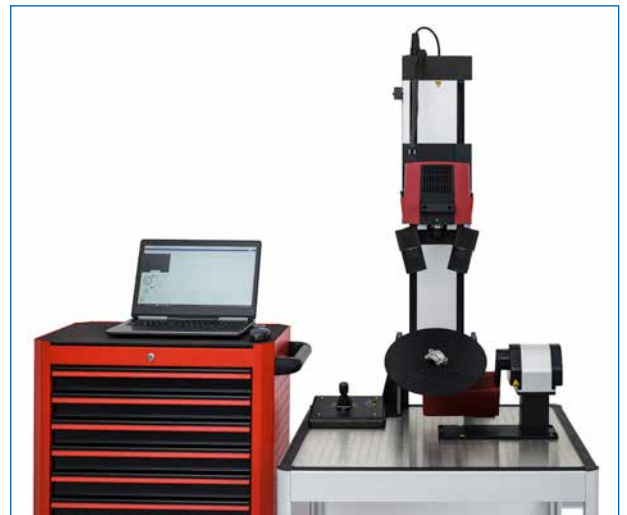
Gom 3D object scanner: digitization of components
